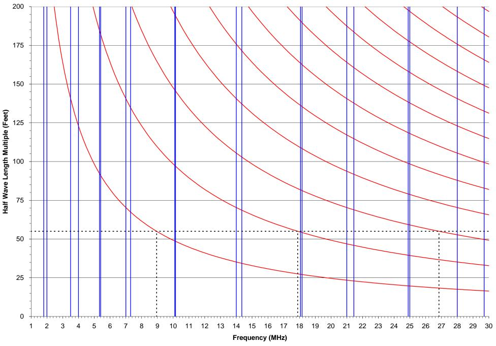
Vertical blue lines indicate US HF amateur band frequency limits. Curved red lines are the half wave integer multiples, in feet, at the indicated frequency.
